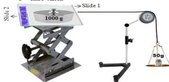
Figure 3. Assembly of spreadability measuring device
